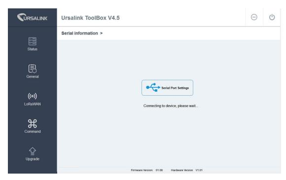
When the Ursalink ToolBox displays: **Connecting to device, please wait...**You can click **Serial Port Settings** to set the correct serial port parameters.
