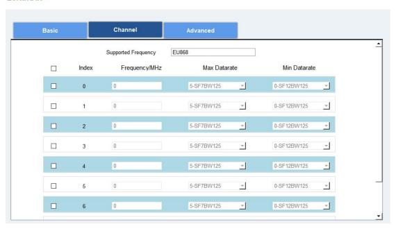
**Note:** Make sure that you have configured the corresponding channel on the gateway. E.g. If you have configured a 923.2 MHz channel on UC1152, then you have to configure a 923.2 MHz channel on gateway as well.
