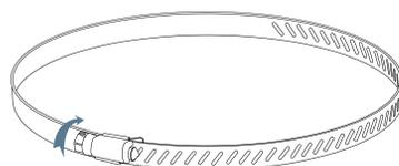
4.Straighten out the hose clamp and slide it through the rectangular holes in the mounting bracket, wrap the hose clamp around the pole.
