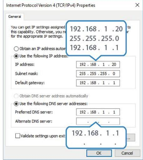
⑤ Double Click “Internet Protocol Version 4 (TCP/IPv4)” to configure IP address and DNS server.
