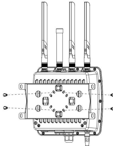
3. Align the mounting bracket horizontally to the desired position on the wall, use a marker pen to mark four mounting holes on the wall, and then remove the mounting bracket from the wall.
